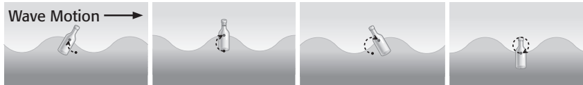
Ocean waves are surface waves. A floating bottle shows the circular motion of particles in a surface wave.
